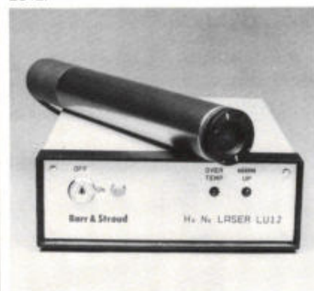
Afb. 8. Barr & Stroud's universele HeNe-laser LU12.
